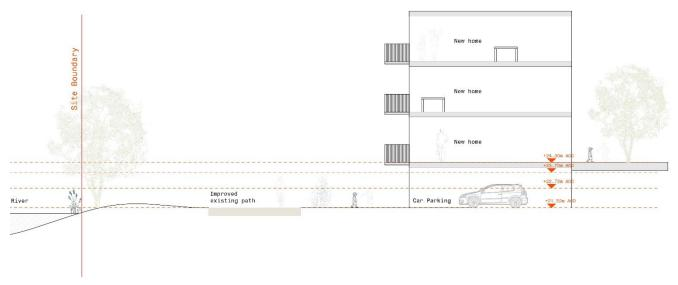
Figure 18: Illustrative section of the river park with a residential building fronting the river. The location of the car park on the ground floor and the new dwelling on the first floor upwards reflects the current masterplan assumptions and highlights the risk of delivering large portions of blank and inactive facades with the new development.
