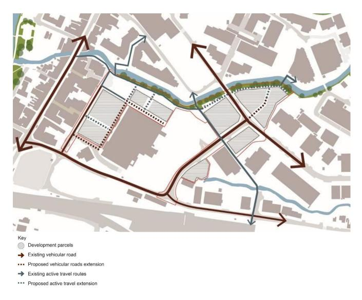
Figure 34: Connectivity and movement diagram.
