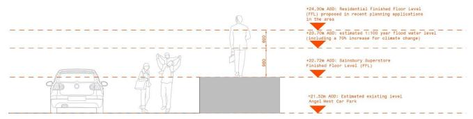
Figure 16 Illustrative section of different ground levels and estimated residential finish floor level (FFL) taken as assumption for the new development.
