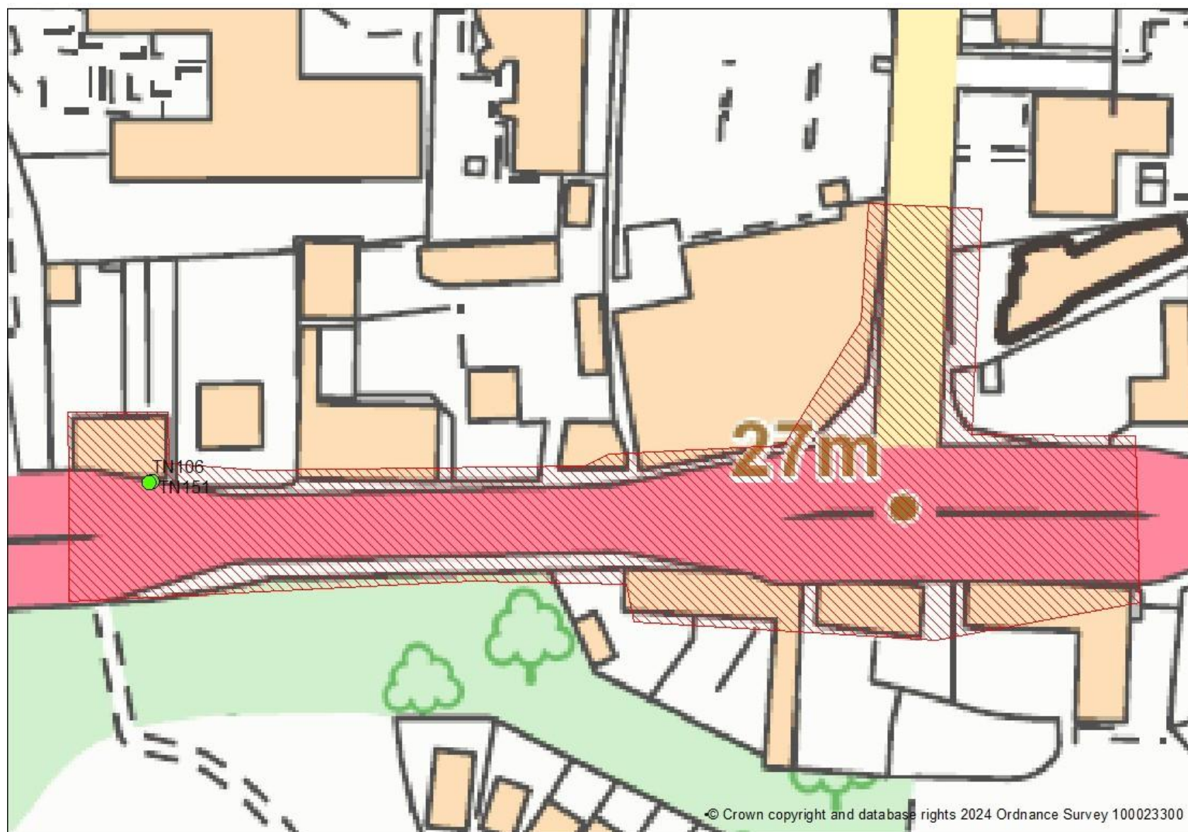
Figure D5 Locations of current and old diffusion tubes for AQMA 6 Larkfield
