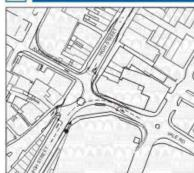
Modified junction layout to deter through traffic from using the high street, design means that drivers are encouraged to undertake a movement. to/from Vale Road. It would be possible to incorporate priority within signals for busses. Potential to create a 'gateway' to the high street.
