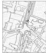
Improvements to junction to deter through traffic from the high street to the outskirts of the town centre. Accompanied by signing structure and visual deterrent of one way road working on High Street. Potential for priority for public transport into/out of the High Street.
